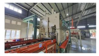
The auto paper lay-up system, auto visual recognition EIR are independently developed by HAPCO's technical team, and has gained a number of China national invention and New utility patents. The precision of the auto EIR reaches an advanced international level!
